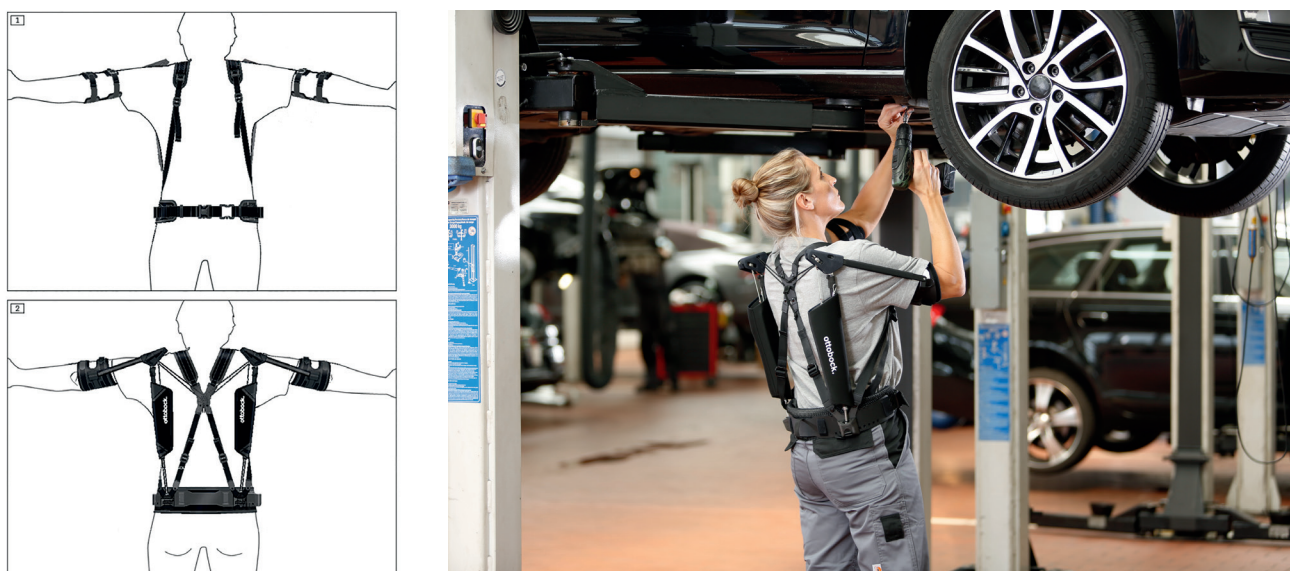
Fig. 1 The exoskeleton used in the front and rear view (left) and for work processes in the automotive industry (right)
